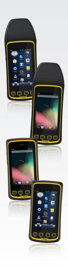
The flexible, fully-rugged Juno T41 is available in a wide variety of configurations. Build the handheld computer you need: Android or Microsoft Windows operating systems, Barcode Imager, Ultra-High Frequency RFID, Smartphone or GPS collector (or combinations). Every Juno T41 is a reliable small workhorse computer designed to last for years in any environment.
